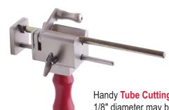
Handy **Tube Cutting Jig** for cutting tubing or rods up to 1/8" diameter may be hand held or secured in a regular bench vise. This heavy duty jig is made of tool steel; the handle is PVC coated. 5½". Weighs 1.25lbs.
